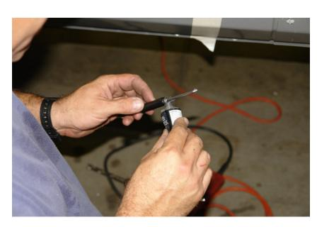
Step 21. Coat the end of the DOM sleeve with a liberal coat of black RTV Silicone before installation.
