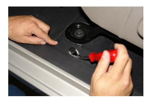
Step 5. Begin to remove interior trim panels to expose inner sill area.
