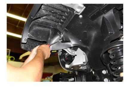
Step 18. Begin to remove inner fender liner clips for removal of inner fender liner
