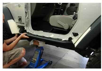
Step 9. Tape the backside of the rail to protect the body of the JEEP, and lift into place.
