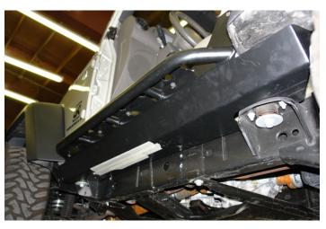
Step 29. After every bolt has been torqued, locate the mounting tabs on each end of the rails. Drill through the hole in the tab with a 1/4" drill bit, and install  $\frac{1}{4}$  -20 x  $\frac{3}{4}$ " hardware
