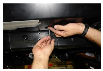
Step 10. Align the holes and bolt the rail into place from the bottom side using the supplied bolts and nut-clips. Use the floor jack out at the end of the tube rail to "cam" or squeeze the rail tightly to body before transferring the hole centers before drilling the body.
