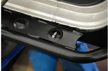
Step 28. After every bolt has been inserted and nuts started on the end of the bolts, begin to torque all of the bolts from the middle mounting points out. Retorque all bolts in sequence twice.
