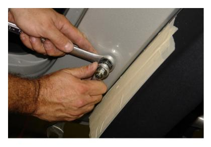
Step 25. Use the supplied tool to install the  $\frac{1}{4}$  -20 nut-sert at the rear upper edge of the rails. **NOTE:** See addendum for 4 door notes.
