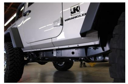
STEP 2. On Sahara & Rubicon models, remove stock step/rock rails.
